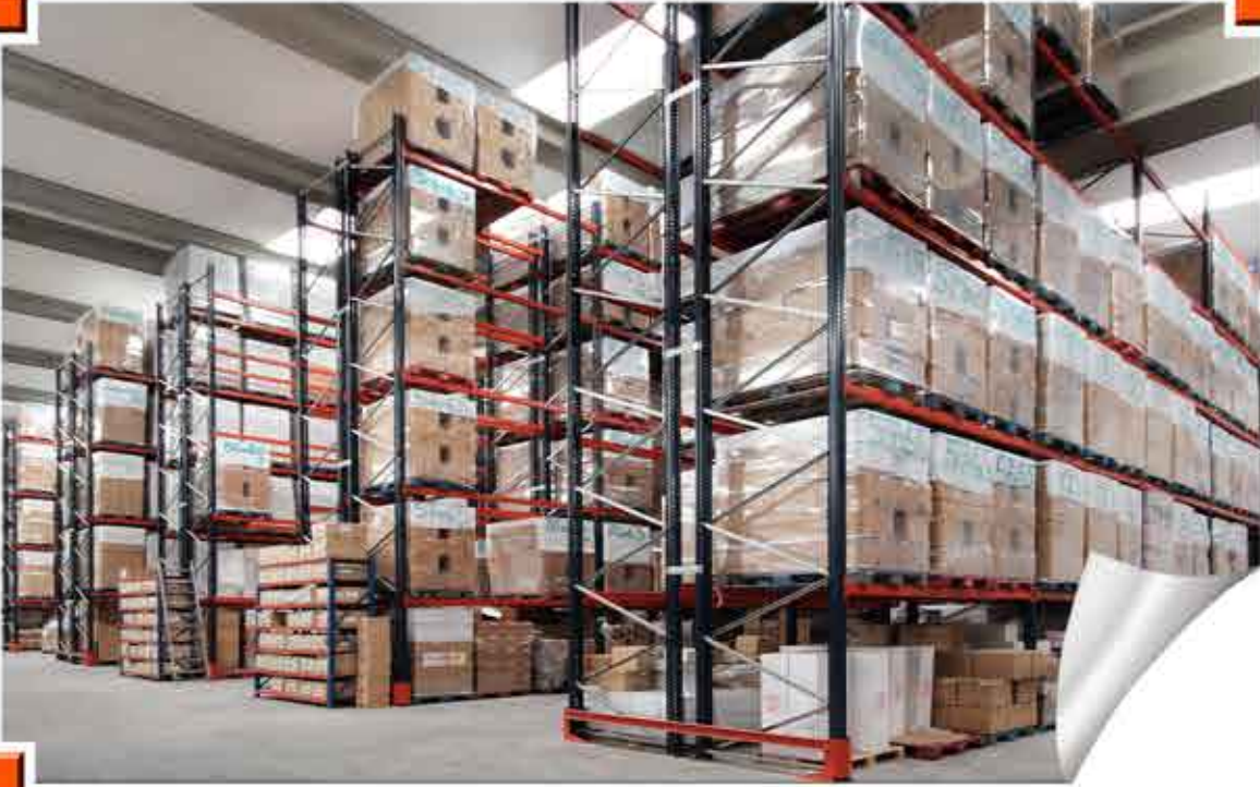
The above image shows a pallet racking warehouse with pallets which are handled by the side measuring 1200mm.
