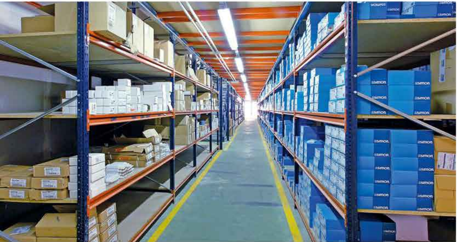
Storage system for manual picking of products following the "man to goods" principle.
